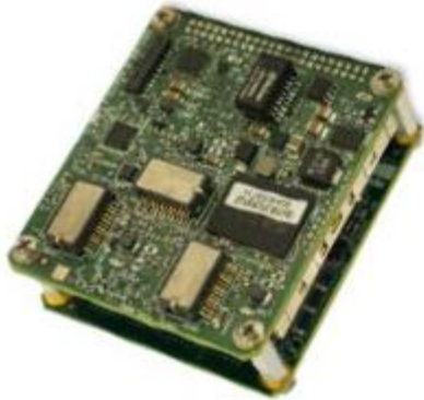
True View 410, 615 APX Board stack contains internal IMU (IMU-59)
